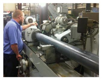
The belt on a belt grinding system is changed by simply stopping the grinder, opening the safety guard door, releasing the pneumatic tension on the belt and removing the belt to be changed. Then reverse the process. Slip the new belt onto the grinding wheel and around the idlers in the belt tensioning system and retension. Close the safety guard door and go back to work. Simple as that.
